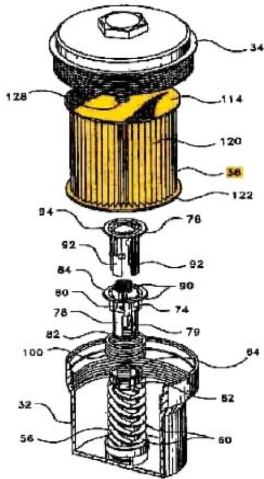
In this Figure, "Figure 3" of the patent, the housing 32 holds a removable filter element 36. The filter element is placed in the housing and an opening in the center of the filter element allows it to slide over support core 56. When the filter element is inserted, the housing cap 34 can be screwed on to close the housing.
