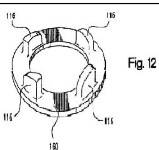
As shown in Figure 12, the "separate annular end piece" is an annular (ring shaped) piece, separate from other pieces that have the protrusions formed into one side of it. Thus, the "separate annular end piece" of the claims of the '426 and '537 patents should be construed to be a stand-alone annular member with protrusions.
