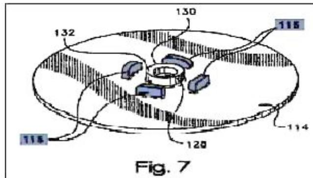
The specification states: "The flange and protrusions can be easily formed with the end cap *such as by molding the end cap as a unitary component....*" (Doc. 139 Ex. 1, '139 patent, col. 4, lines 4-6 (emphasis added).) Wix argues that the annular flange is always shown, or "embodied," as formed from a single piece with top end cap.
