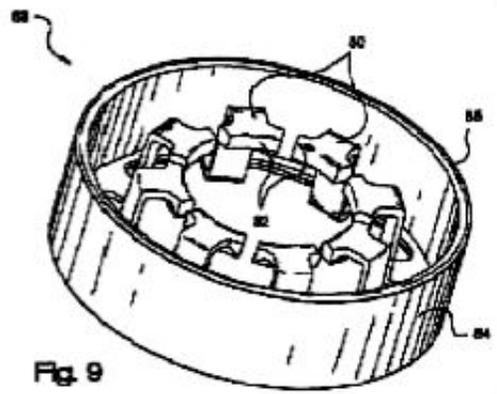
The valve device 64 (shown in Figure 8 above) includes base 72. Tabs 76 extend outwardly from the sleeve, and define a series of slots 78. The latch 68 includes fingers 80, each of which has radially-inward ends 82. The fingers are forced slightly outwardly when the latch is in the locked position. The latch is located between the valve and the lower end of the filter housing as shown in Figures 3 and 4.
