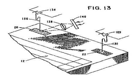
The patent explains that this configuration, in which both LEDs (labeled 129 and 134 in Figure 13) are on the I Module and data is transmitted by the P Terminal using reflection, allows the non-portable I Module to provide the power to the LEDs so that the smaller, battery-powered P Terminal is more energy-efficient.
