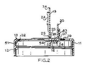
Returning to the '494 patent, Figures 2 and 5-8, shown below, also clearly show that the "land 36" is anchored to the inner wall of skirt 11 by ribs 71. These ribs, together with the skirt and the land, create a series of arcuate, box-like structures. According to the specification, that connection imparts greater rigidity to the cap:
